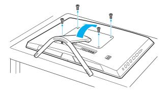
**3** Remove the 19 screws (1) from the back of the foot stand and take off the mounting base plate (2).
